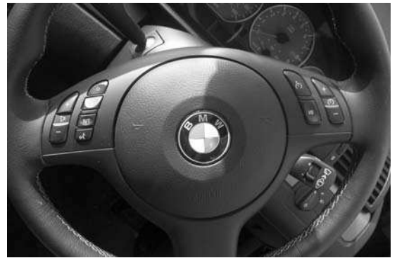
Figure 9.63 Supplementary restraint system (SRS) – an air bag is incorporated in this steering wheel
