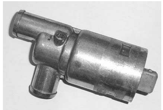
Figure 4.31 Rotary idle speed control valve
