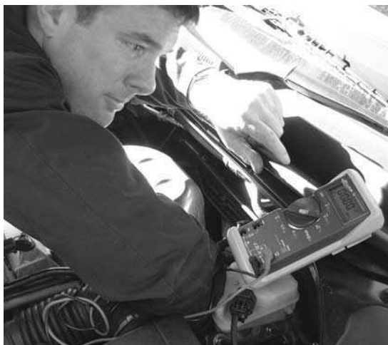
Figure 9.56 Circuit voltage testing
