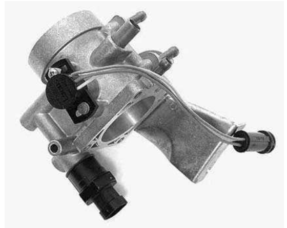
Figure 4.33 Stepper motor and throttle potentiometer on a throttle body
