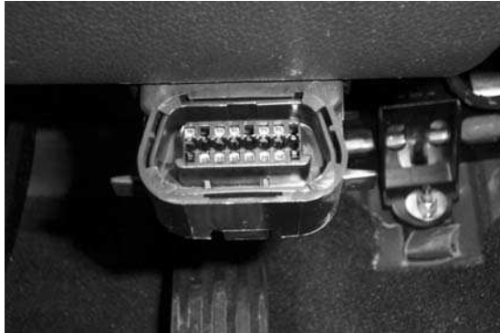
Figure 4.45 OBD socket – pin 6 is CAN-high and pin 14 is CAN-low
