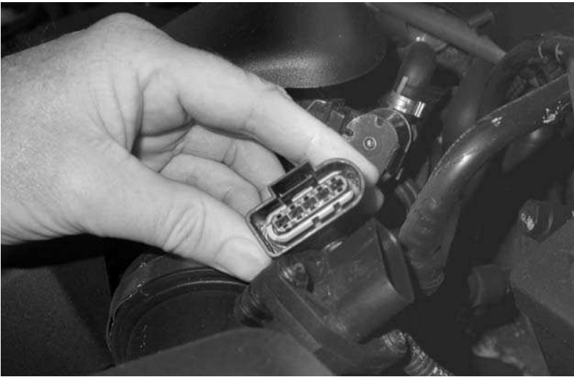
Figure 7.43 Air flow meter under test
