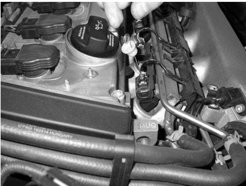
Figure 2.6 Test the voltage at a connection with care
