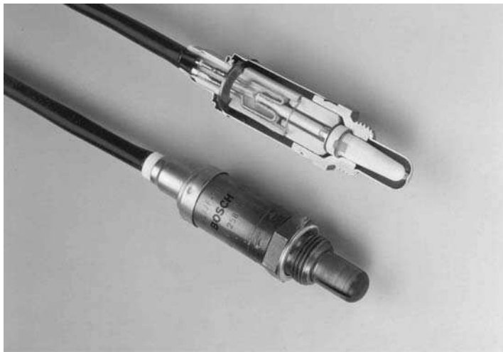
Figure 4.18 Zirconia type oxygen sensor
