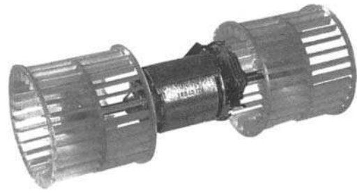
Figure 9.49 Heating and ventilation motor and fans
