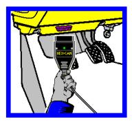
◄ If your vehicle has a 2x2 port (some pre-1996 vehicles), then use the optional 2x2 Adapter between the Interface and the ports in the car. This is included in the Pro-Kit.
